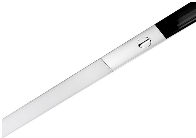
Linear lighting module for electrified track for interiors, with direct light emission. Structure in anodized extruded aluminium. Extruded polycarbonate diffuser with opaline finish. End caps in black thermoplastic material with fixing system for 48V low voltage electrified tracks.
