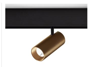
Lighting fixture for electrified track for interiors, with swivelling light beam. Die-cast aluminium joint and double-axes rotating structure.
