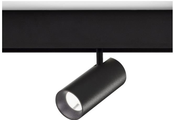
Lighting fixture for electrified track for interiors, with swivelling light beam. Die-cast aluminium joint and double-axes rotating structure. Thermoplastic anti-glare snoot and medium-beam lens. Equipped with electric and mechanical adapter for 48V low voltage electrified tracks. Available in 2700K and 3000K version, in white, black, mat brass, bronze and titanium finishes, with black arm and back cover.
