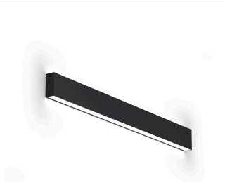
Wall lighting fixture for interiors, with direct and indirect light emission. Extruded aluminium structure in RAL 9003 white or black powder paint. Extruded polycarbonate diffusers with opaline finish. Pickled sheet metal end caps in polyacrylic paint. Equipped with wiring for separate switches for direct only, indirect only or direct and indirect light emission.
