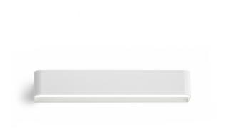
Wall lighting fixture for interiors, with direct and indirect light emission. Body in extruded aluminium and cover in pickled sheet steel, with white, black, bronze, mat brass or titanium polyacrylic paint. Wall mounting bracket in bent steel sheet. Opal polycarbonate diffuser screens.
