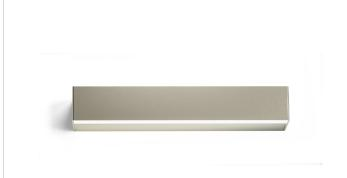
Wall lighting fixture for interiors, with direct and indirect light emission. Body in extruded aluminium and cover in pickled sheet steel, with white, black, bronze,  $\,$ mat brass or titanium polyacrylic paint.
