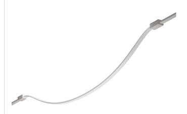
Flexible electrified profile for wall and ceiling installation for interiors. Structure in polycarbonate extruded in mat black or wood finish. 24V DC low voltage power supply. Complete with 4 fixing boxes and 1 power supply kit. Led module to be ordered separately. Length: 3,05m (120,1").
