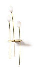
Light fixture for indoor wall installation with diffuse emission. Steel, aluminum and brass structure. No.3 blown glass diffusers with diffusing finish. Wall mounting base made of galvanized sheet metal. Polyacrylic paint in mat black or mat brass color. Max 3x 4W G9. Dimmable G9 2700K LED sources included.
