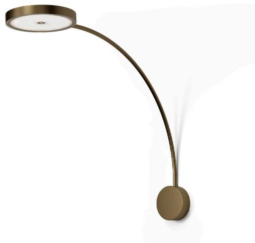
Wall installation lighting fixture for interiors, with direct or indirect light emission. Power supply canopy with pickled sheet metal fixing bracket, deep-drawn sheet metal closing frame in polyacrylic paint. Calendered steel tube stem, with polyacrylic paint. Die-cast aluminum emitting head with polyacrylic paint in champagne, mat black, bronze and soft textured white finishes. UV technology screen-printed diffuser, made of opal polycarbonate, installed with magnetic coupling.
