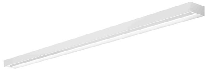
Ceiling or wall lighting fixture for interiors, with direct and indirect light emission. Pickled sheet metal structure in white, bronze or mat brass polyacrylic paint, or with gold leaf coating, or in polished stainless steel. Specular aluminium reflector. Cover in brass with white, bronze or mat brass polyacrylic paint, or with gold leaf coating, or with galvanic chrome plating. Extruded polycarbonate diffuser with opaline finish.
