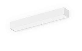
Wall lighting fixture for interiors, with direct and indirect light emission. Pickled sheet metal structure in polyacrylic paint. Aluminium dissipation plates. Pickled sheet metal cover in white, bronze or mat brass polyacrylic paint, or with gold leaf coating, or in polished or mat stainless steel.
